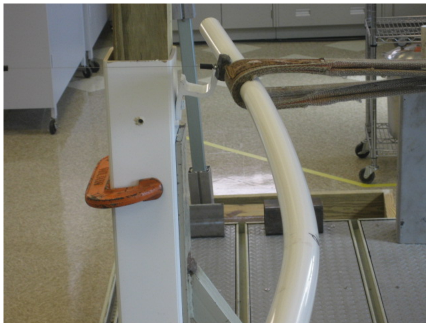
Photo No. 2 Concentrated Horizontal Load Test at Ends of Handrail (Bracket)
