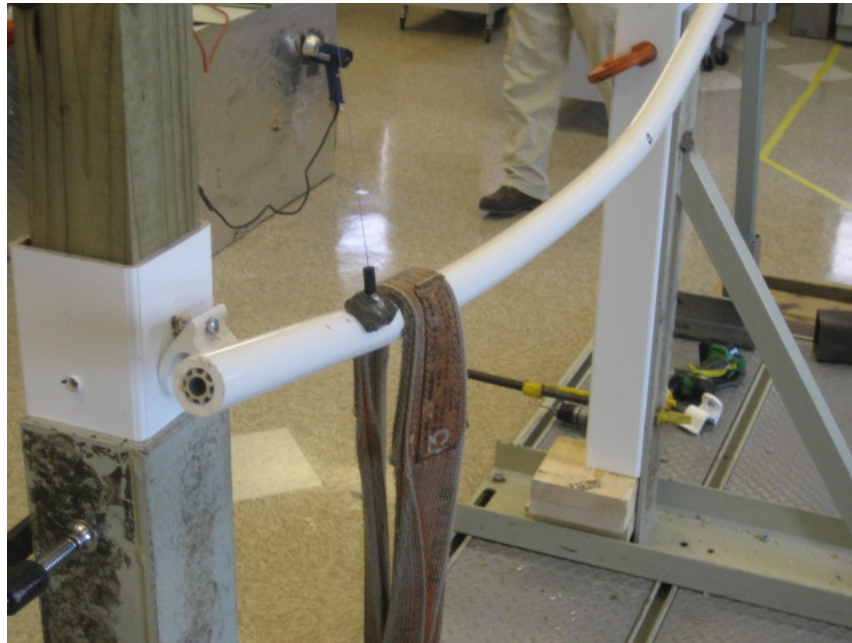
Photo No. 3 Concentrated Vertical Load Test at Ends of Handrail (Bracket)
