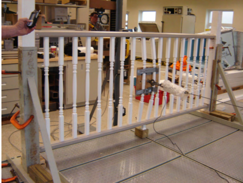
Photo No. 1 Infill Loading at Center of Balusters
