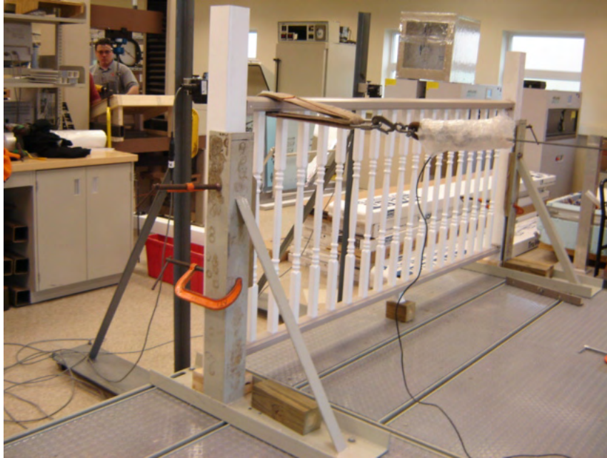
Photo No. 3 Concentrated Load at End of Rail (Bracket)
